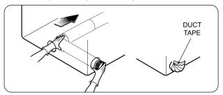
**3-2.** Insert elbow duct assembly first through the side opening and connect the elbow to the internal duct.
